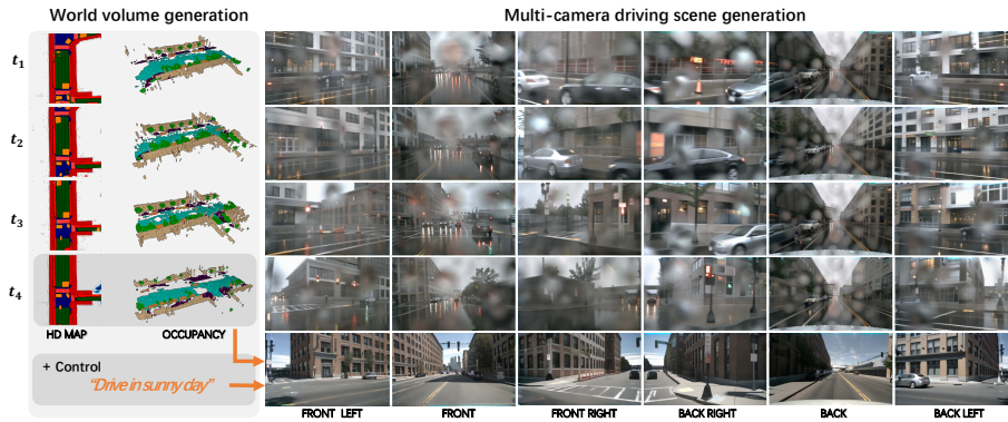
Fig. 1: Our WoVoGen is crafted to generate future world volumes ( i.e. , HD maps and occupancy) and high-quality multi-camera street-view images, with the input of past world-volumes. The bottom row shows the weather-based control of WoVoGen. Specifically, with the predicted world volume at time t_4 and a weather description, the multi-camera images transit from rainy to sunny conditions, while maintaining the street layout.
